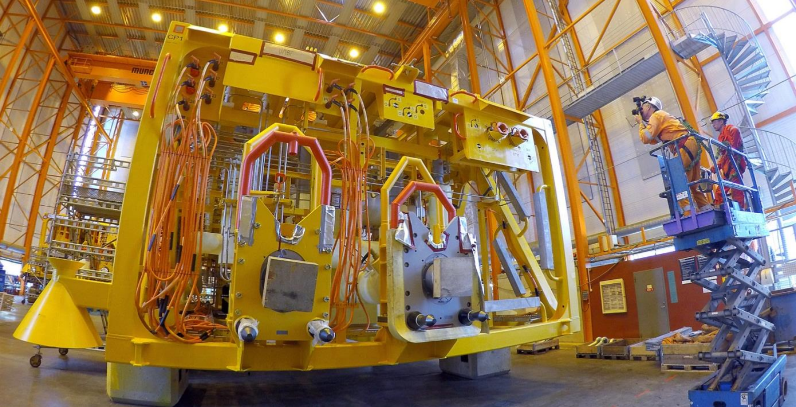
Photogrammetry dimensional control survey of a manifold – Fugro 2016
